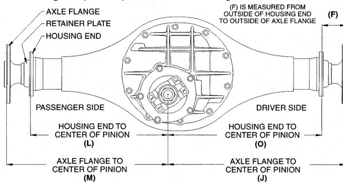
NOTES: (1) Axle Flange to Axle Flange is measured from the OUTSIDE (Wheel Side) of the axle's flange to OUTSIDE (Wheel Side) of the opposite axle's flange. (2) If you have listed only housing end to housing end or axle flange to axle flange- you must specify pinion offset.
