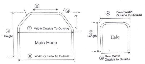
Please make main hoop measurements at doorpost area A: Measure at headliner, where it rolls down at finish trim molding D: From headliner down to door, where window rolls down into Halo: Measure in visor area on roof
